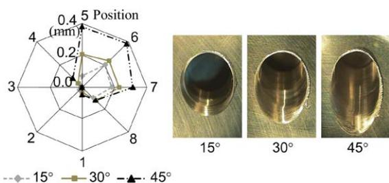
Fig. 2. Result of deburring experiment with Burr-Off tool with Al6061 under the following conditions: inclination angle of 15°, 30°, and 45°; spindle speed of 700 rpm; feed rate of 28 mm/min; diameter of 9 mm; with coolant.
