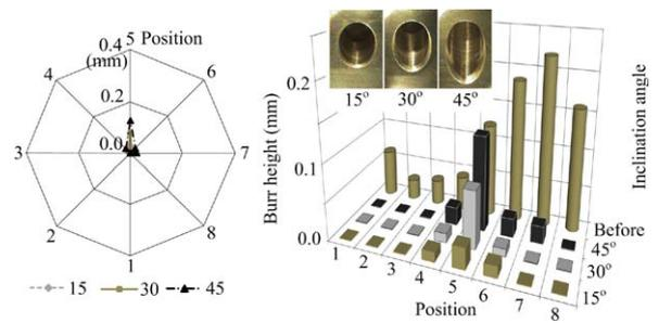
Fig. 6. Result of the deburring experiment using tool 2 with inclination angles of 15°, 30°, and 45°; a speed of 700 rpm; a feed rate of 28 mm/min; a diameter of 9 mm; and using Method 4.
