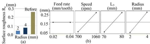
Fig. 8. Change of surface roughness according to the change of (a) radius of tool tip, (b) some parameters.
