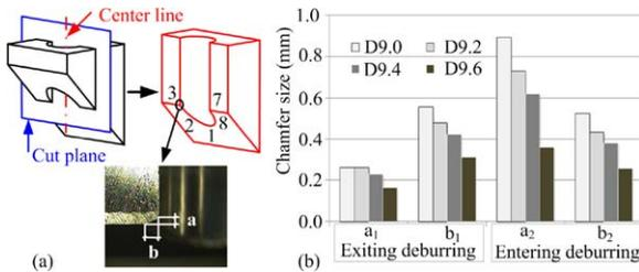
Fig. 9. (a) Definition of cutting plane and chamfer size. (b) Chamfer size of drilled hole after deburring with exiting deburring ( $a_1$ ,  $b_1$ ), entering deburring ( $a_2$ ,  $b_2$ ), tool 2, a spindle speed of 700 rpm, a feed rate of 28 mm/min, and an inclination angle of 15°.
