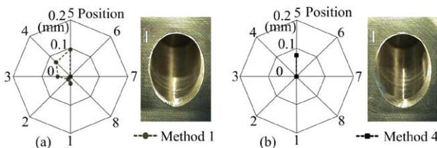
Fig. 5. Burr size after deburring with tool 2 at a spindle speed of 700 rpm, a feed rate of 28 mm/min, an inclination angle of 30°, and with coolant using (a) deburring Method 1 and (b) deburring Method 4.
