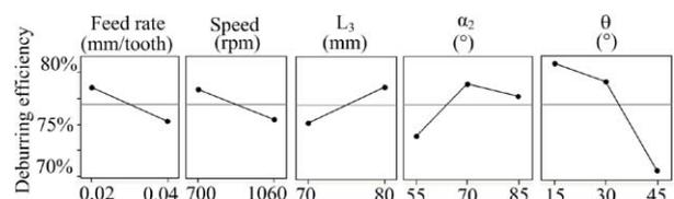
Fig. 7. Change of deburring efficiency according to the change of parameters.
