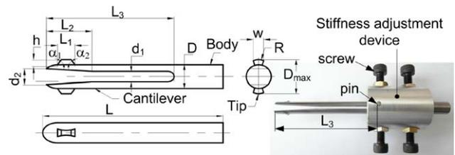
Fig. 3. Deburring tool geometry and stiffness adjustment device.
