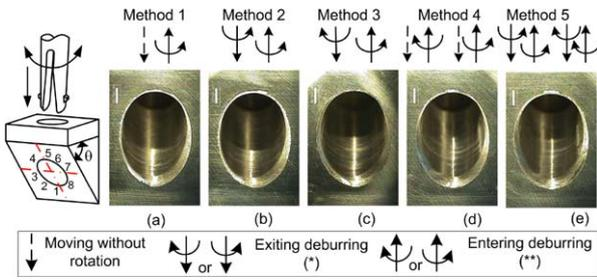
Fig. 4. Deburring experiment results using different methods. (a) Method 1, (b) Method 2, (c) Method 3, (d) Method 4, and (e) Method 5.
