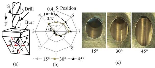
Fig. 1. Burr formation with different inclination angles with respect to the exit surface for aluminum (Al6061), a speed of 800 m/min, a feed rate of 100 mm/min, and dry conditions.
